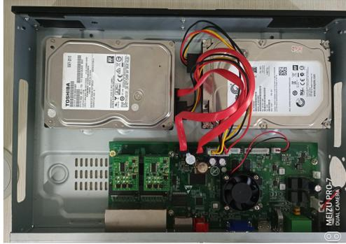
Figure 1-7 Connecting the Cable
