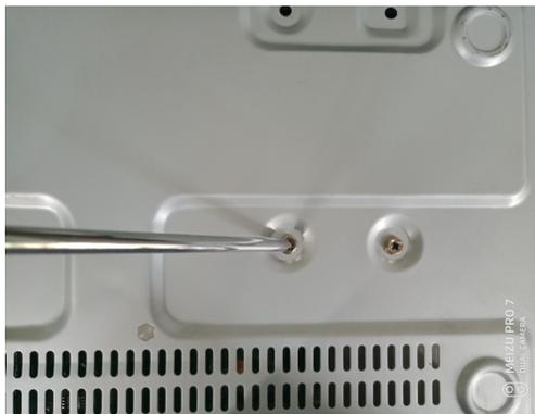
Figure 1-6 Fasten the hard disk
