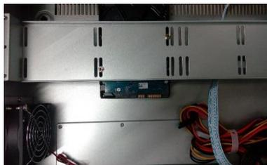
Figure 1-2 fasten the hard disk
