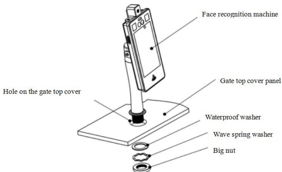
**Note: Roof opening size of gate machine is  $\text{Ø } 40 \text{ mm } (+ / - 2)$ .**
