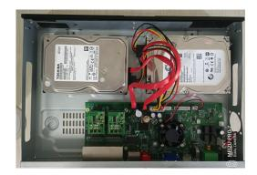
Figure 1-7 Connecting the Cable
