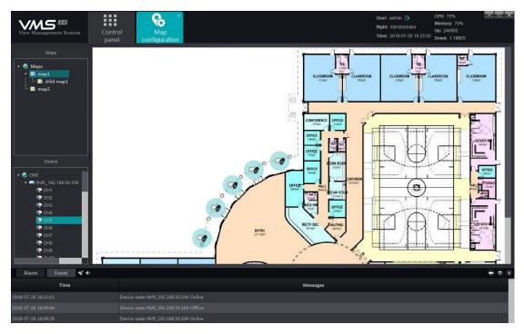
Note: as the channel has been dragged to the map, the position shall be adjusted by dragging it again; right click on the deployed channel, it shall be deleted. Place the mouse on the map, scroll the wheel can zoom in/zoom out the map. The channel deployed to the map shall not be dragged repeatedly, and place the mouse on the deployed channel, the channel information shows.
