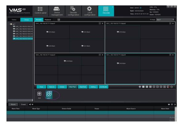
Configure the pre-arranged plan, select the decoder split screen, decoding stream type and channel to edit the plan, edit completed, click "save the plan", complete the editing.
