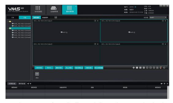
Drag to the output group of TV wall, will automatically open the group round touring, the round touring time interval can be set when configuring decoding group, the default is 20S.
