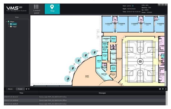
Double-click the map, you can display the configured map and layout channel, this module is an operation module, can not configure and modify map, right-click the layout channel, can open the preview and playback of the corresponding channel. In actual use, the user can refer the map, quickly pick up the preview and playback image of the corresponding location, more concise and clear operation. The channel icon flashes when an alarm is triggered and the linkage channel is on the map.
